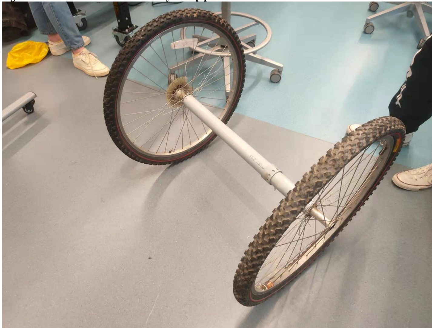
Figure F1. Two-wheel axles combined by PVC pipes
