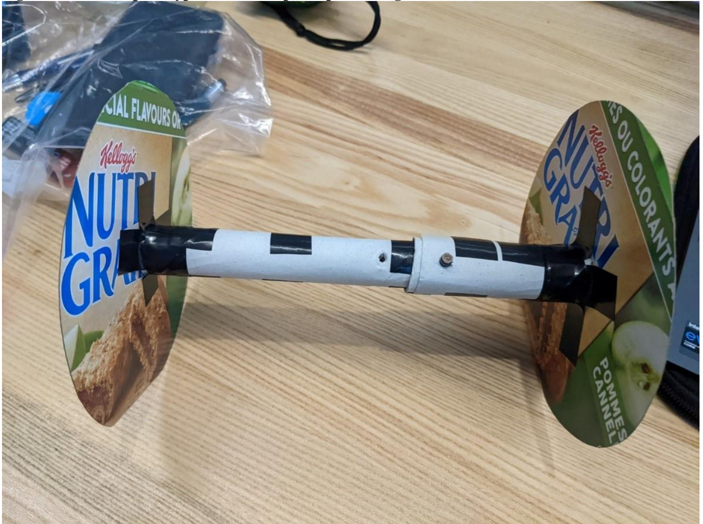
Figure E14: Initial prototype of axle set up and pin locking mechanism
