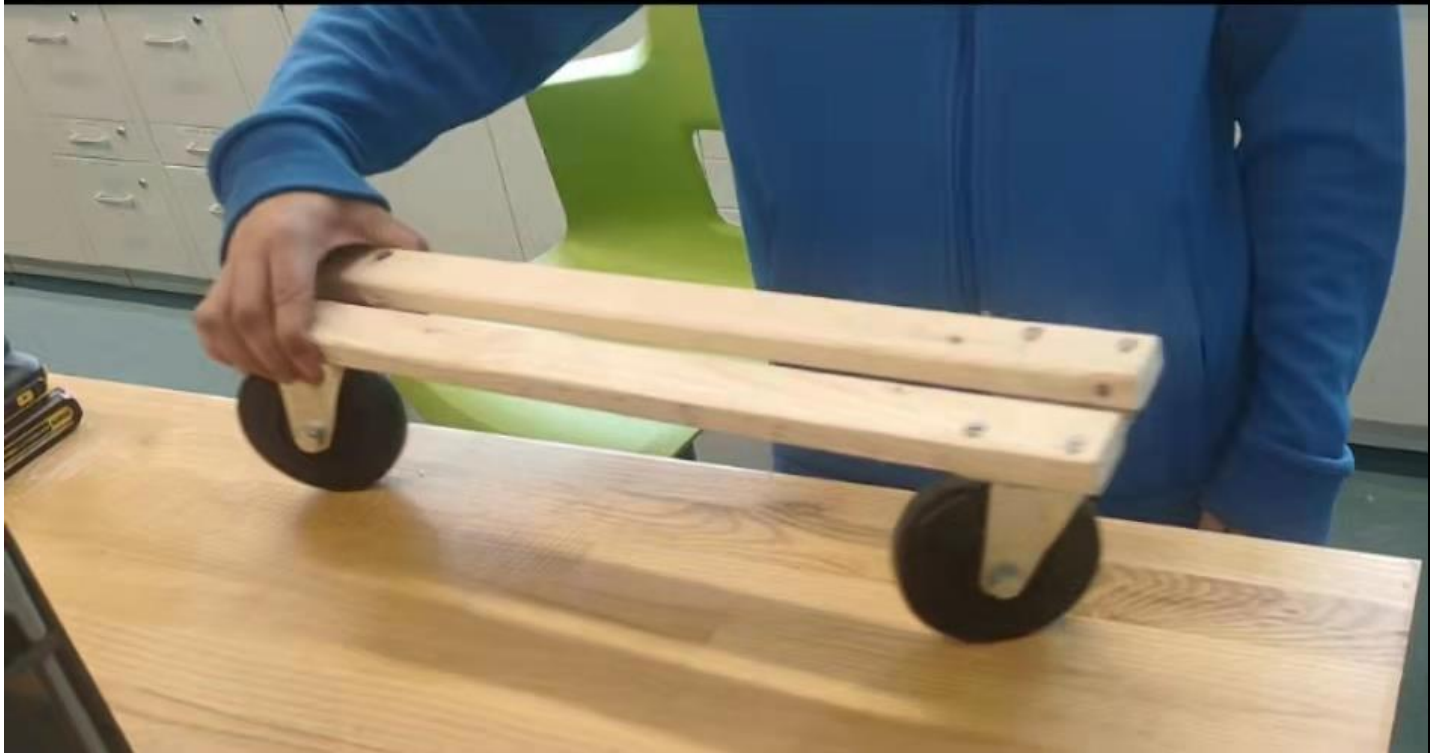
Figure F2. Connecting the casters with pins and planks
